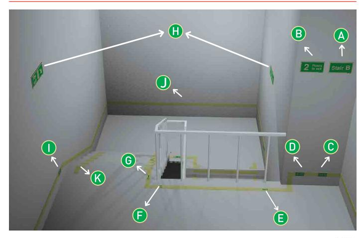
A Rigid plastic stairwell signs - ③ Everlux<sup>\*</sup> - To be installed at the High Location level (above 1.8m) - refer to Pg. 94 for details
