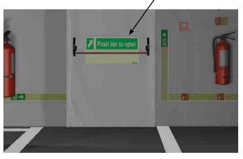
The emergency exit opens on the right hand side and this is indicated by the signs and strips being positioned to the right and parallel to the door opening mechanism.
