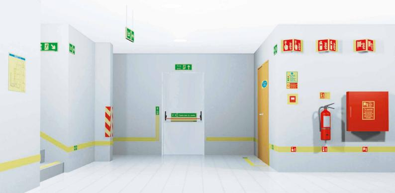
This image provides a guide on fire signage and safety requirements, and placement of relevant signs.
